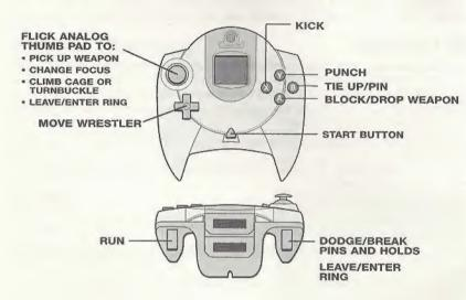
Never touch the Analog Thumb Pad or Triggers L/R while turning the Sega Dreamcast power ON. Doing so may disrupt the controller initialization procedure and result in malfunction.
